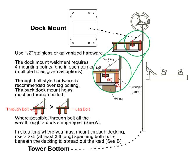
Tower bottom **MUST** be mounted to the dock, dock support structure or to the ground.
