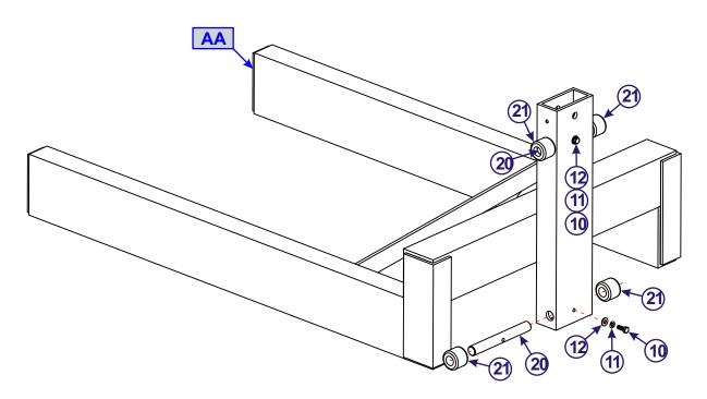
Apply a small amount of anti-seize inside of rollers prior to placing on axle
